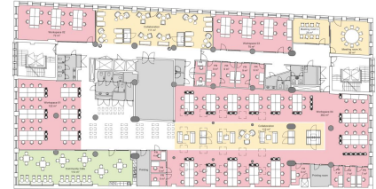
Workstations: 134 x 180cm = Total 134 WS Workstations: 4 Meeting Room: L: 1 Meeting Room: S: 1 Focus Room: 2 Printing Room: 2
